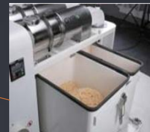
Dust bin inside the machine
