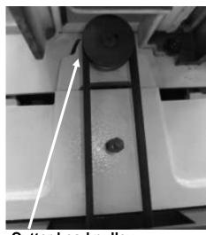
Cutter head pulley
