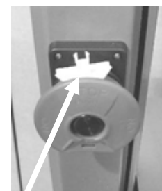
Start/stop with safety removed
