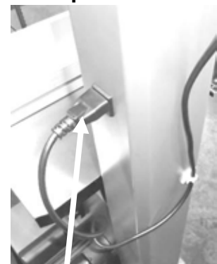
Light plugged into 110v socket
