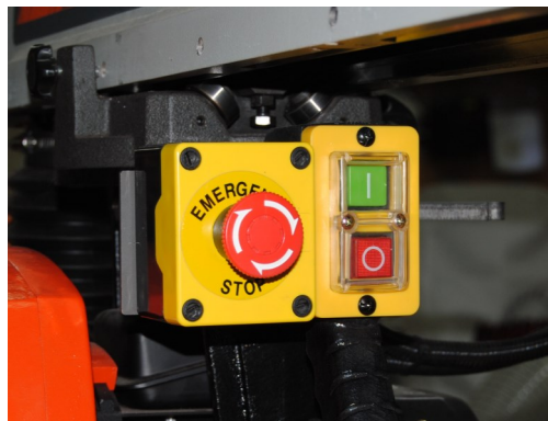
Emergency stop mounted at front side of machine
