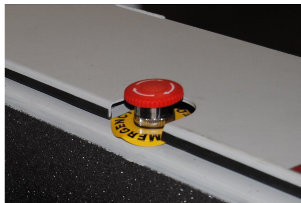
Universal emergency stop that can be activated in both operating positions
