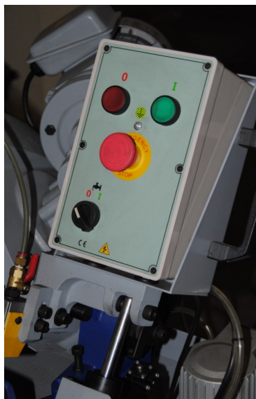
Front mounted emergency stop
