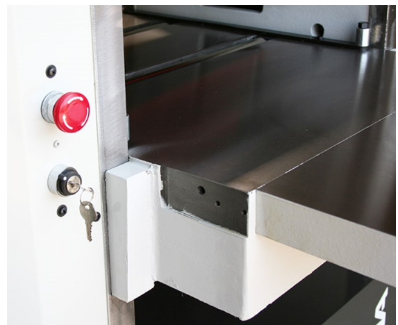
Front mounted emergency stop and key lock out
