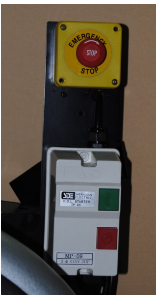
Top mounted emergency stop
